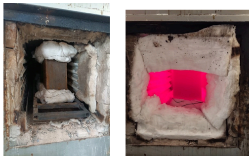
Figure 4 Fire exposure of CFST specimens in furnace
