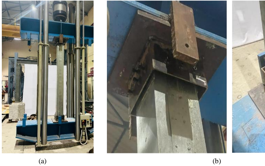
Fig. 4. (a) Experimental test set-up for axial load testing of CFSTC sections; and (b) boundary end conditions for CFSTC sections at the top and bottom respectively.
