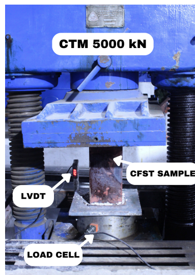
Figure 5 Experimental view of the test setup
