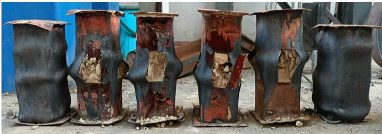
Figure 6 Failure modes of column specimens
