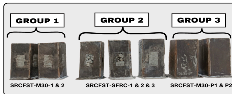
Figure 2 Stub column specimens casted
