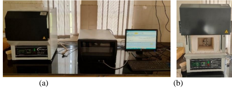
Fig. 3. TPS hot disk setup for evaluating thermal property of concrete
