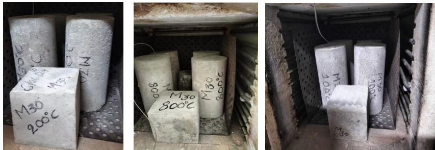
Fig. 5. Fire exposure of specimens in muffle furnace
